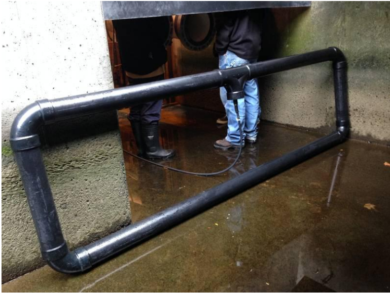
Figure 2. Antenna placed at entrance to BON AFF channel during noise listening survey conducted in fall 2013. This location was rejected due to possible flow disruption and fish strikes.
