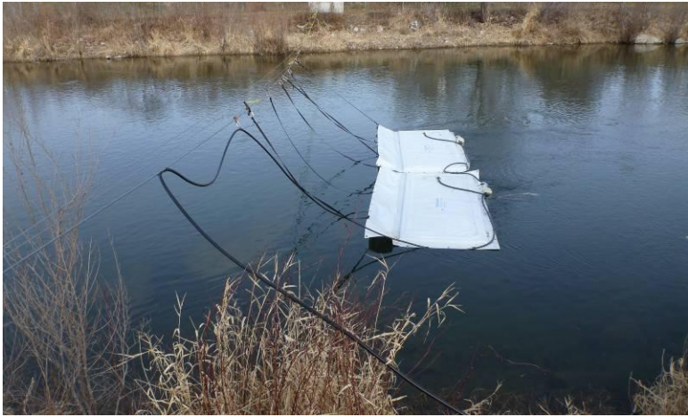
Figure 6. Picture of 2-10' BIO Float antennas installed in the Okanagan River, BC in spring 2014.
